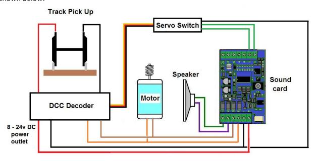
Many decoders also have function outputs which can be used to trigger sounds. However, this is
