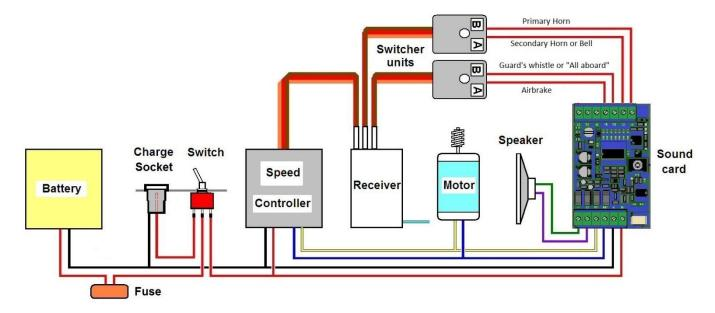
The receiver shown has two function channels, each of which can operate two triggers via two switcher units. The fifth soundcard trigger, the turbocharger, therefore cannot be radio controlled and will need to be switched on, if required, by the IR remote control. A suitable switcher unit is the Pololu 2802.
