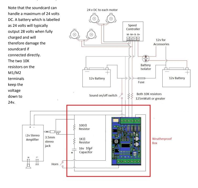
In Australia, the 2x15 watt AA0487 amplifier from Jaycar is suitable. Other amplifiers may require the  $100\Omega$  resistor to be changed. If the output volume is too low then raise the value of the  $100\Omega$  resistor.
